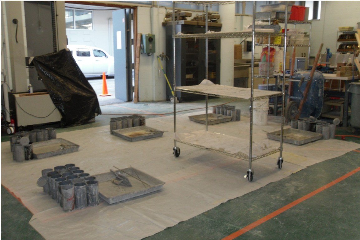
Figure B-1 - Setup for concrete mixing
