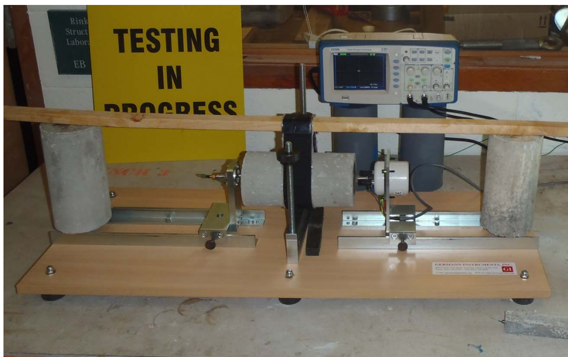
Figure B-12 - Fundamental longitudinal resonant frequency testing
