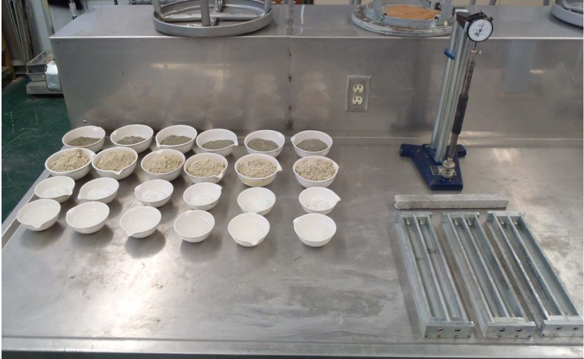
Figure A-1 - Setup for mixing ASR specimens
