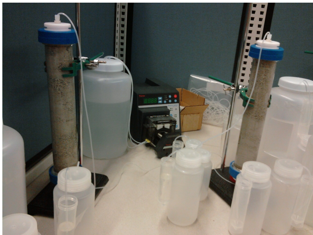
Figure A-9 - EPA Draft Method 1314 Percolation Column setup closeup
