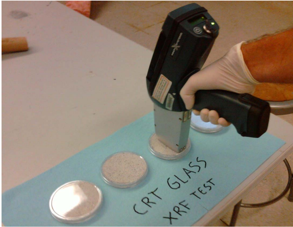
Figure C-1 - XRF testing of CRT glass
