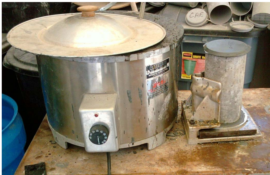
Figure A-4 - Sulfur capping specimens for Compressive Strength Test
