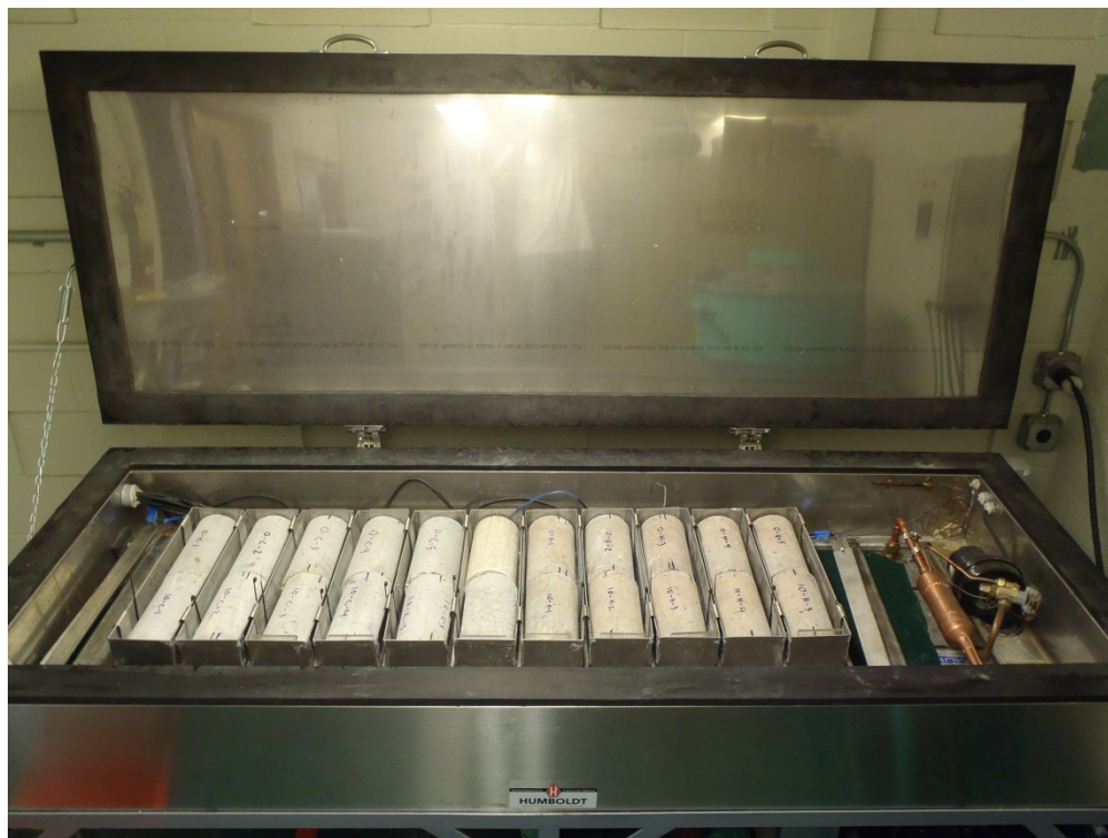
Figure B-8 - Freeze / Thaw testing setup
