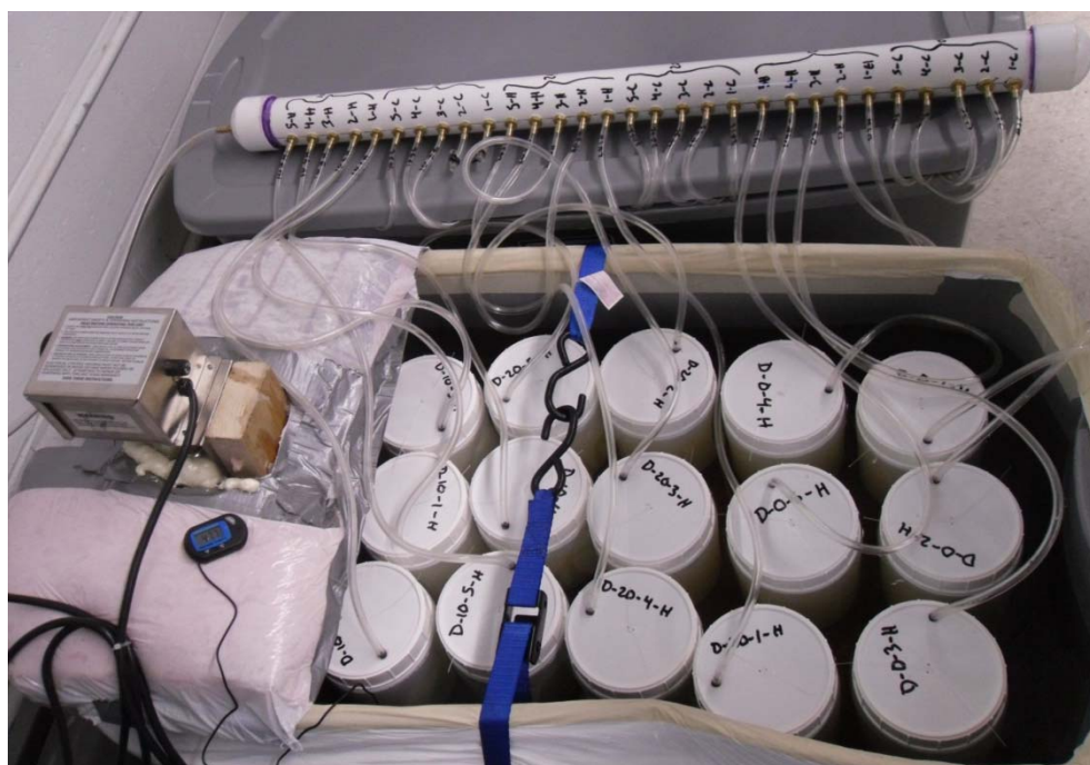
Figure C-3 - Modified diffusion leaching test setup
