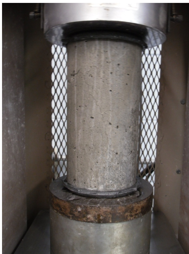
Figure A-5 - Compressive Strength Test
