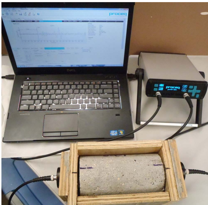
Figure B-10 - UPV testing equipment
