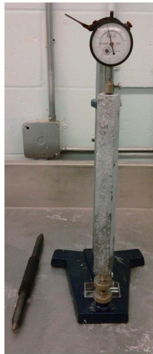
Figure A-3 - ASR specimen being measured
